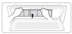
To assemble the air filter, proceed in reverse order of detaching.
