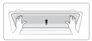
**4** Resetting the air filter (Wired remote control is an optional item.)
