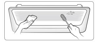
Wipe the surface of the indoor unit with a tepid damp cloth.
