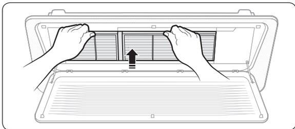
To assemble the air filter, proceed in reverse order of detaching.
