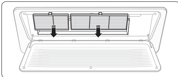
Pull the air filter out of the indoor unit.
